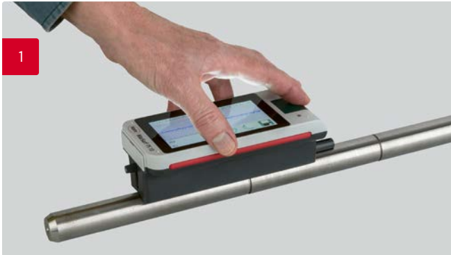
1. Roughness measurement on shafts
