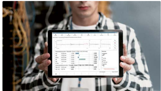
Section from the “RoughnessPlus” section. Virtual rulers to interactively set distances in X and Z direction in the profile field
