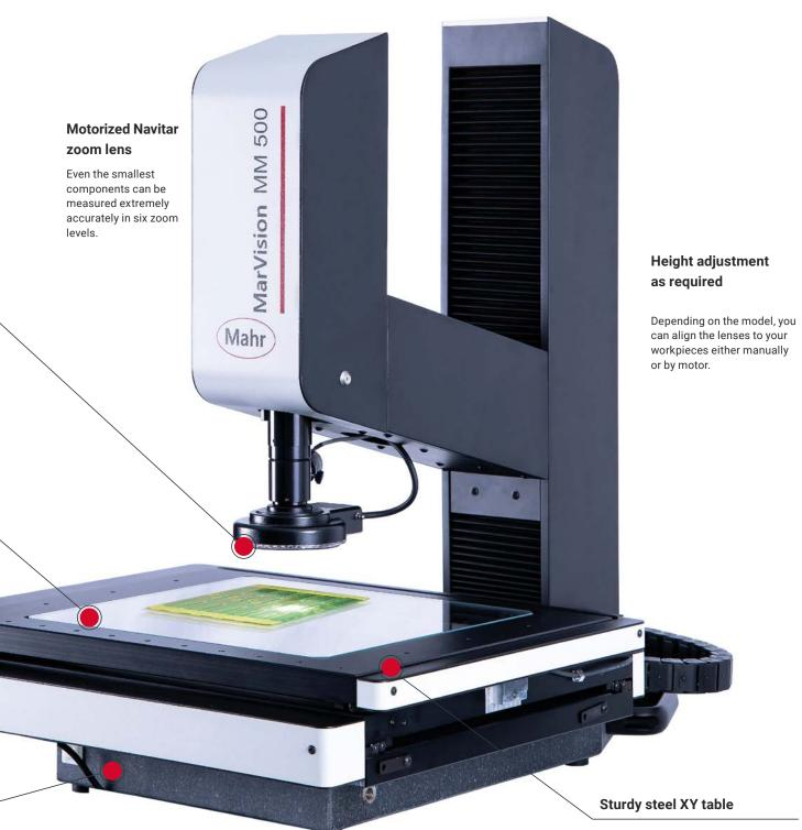
This provides the ideal support, even for delicate workpieces, and enables perfect working with incident and transmitted light.
