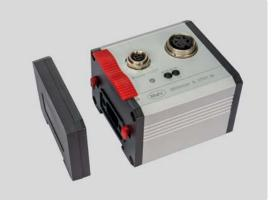
Equipped with an input for inductive probes, the Millimar A 1701 M picks up the incoming carrier frequency signal and converts it to a standardized analog signal, for example ±10 volts or 0 to 10 volts. An LED display provides you with information on the operating status at all times. The compact and robust housing facilitates use in production environments and can be mounted on a rail if required.
