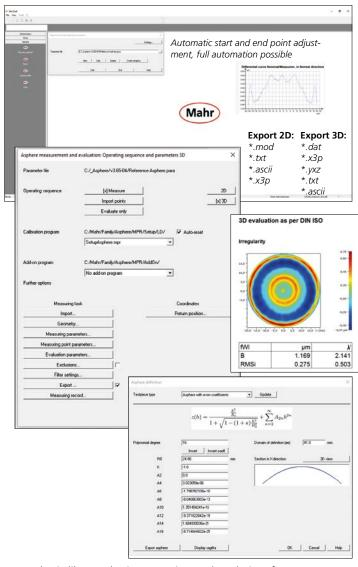
Aspheric.lib - Aspheric measuring and analysis software
