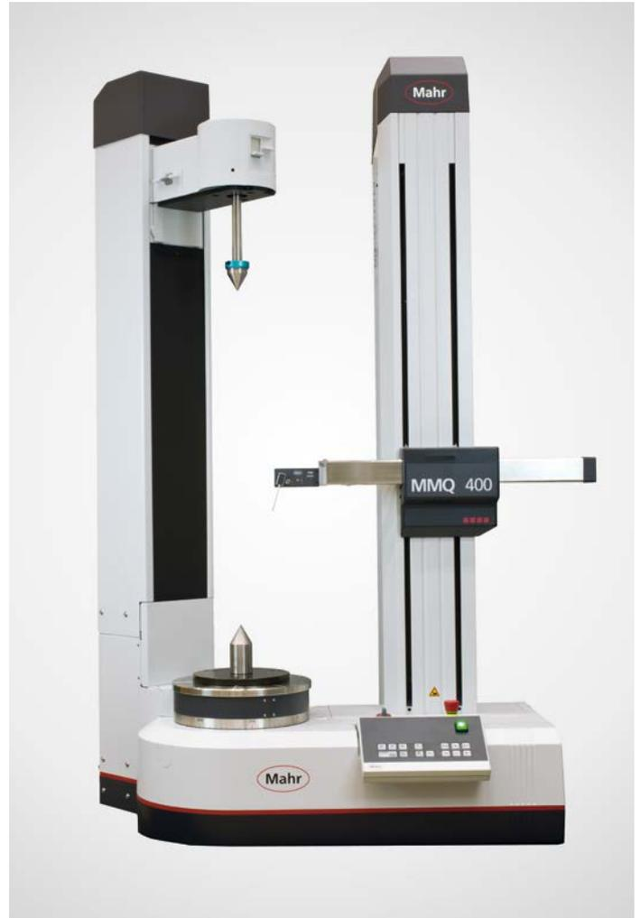
The motorized tailstock and the motor-driven CNC centering and tilting table can be operated alternately, thus increasing the already high flexibility of MarForm MMQ 400 and widening its amazing range of applications even further.
