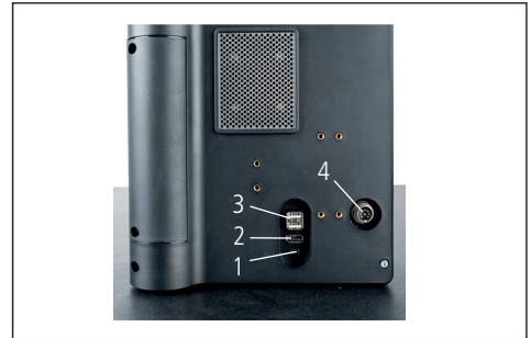
Fig. 9 USB sockets 1 Mini USB 2 1 x USB 3.1 (black) 3 2 x USB 3.1 (white) 4 8-pin round plug for powering the control panel
