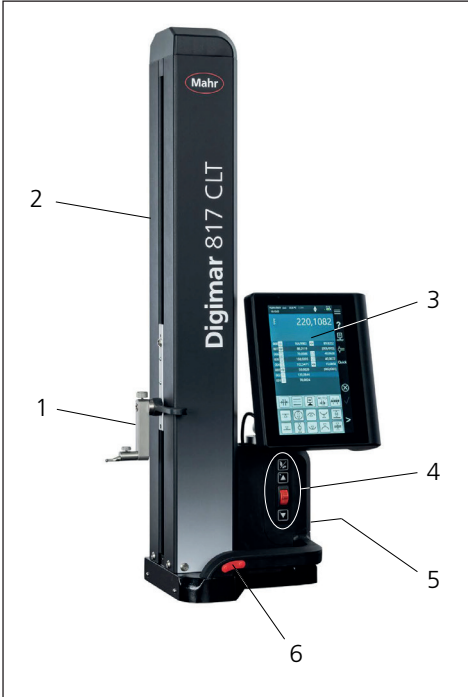
Fig. 1 Elements of the height measuring instrument (The image shows the Digimar 817 CLT.)
