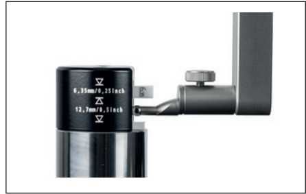
Fig. 12 Positioning the setting gage when calibrating with groove
