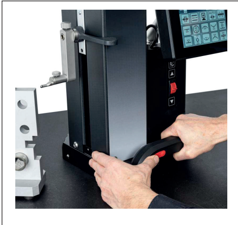
Fig. 7 Moving the height measuring instrument using the activated air bearing (The image shows the Digimar 8127 CLT.)
